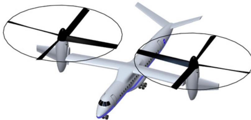
**Figure 4:** NASA Large Civil TiltRotor concept [Acree, 2012]
